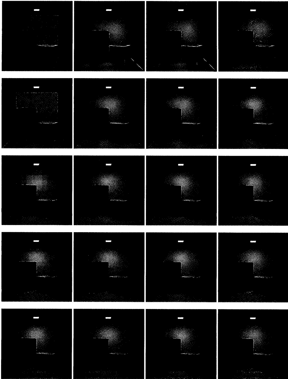
Figure 13. Final rendered images. From left to right: AM-C , AM-H , FOSE , NEW . From top to bottom: 10^3 , 10^4 , 10^5 , 10^6 , and 10^7 particles are traced.
